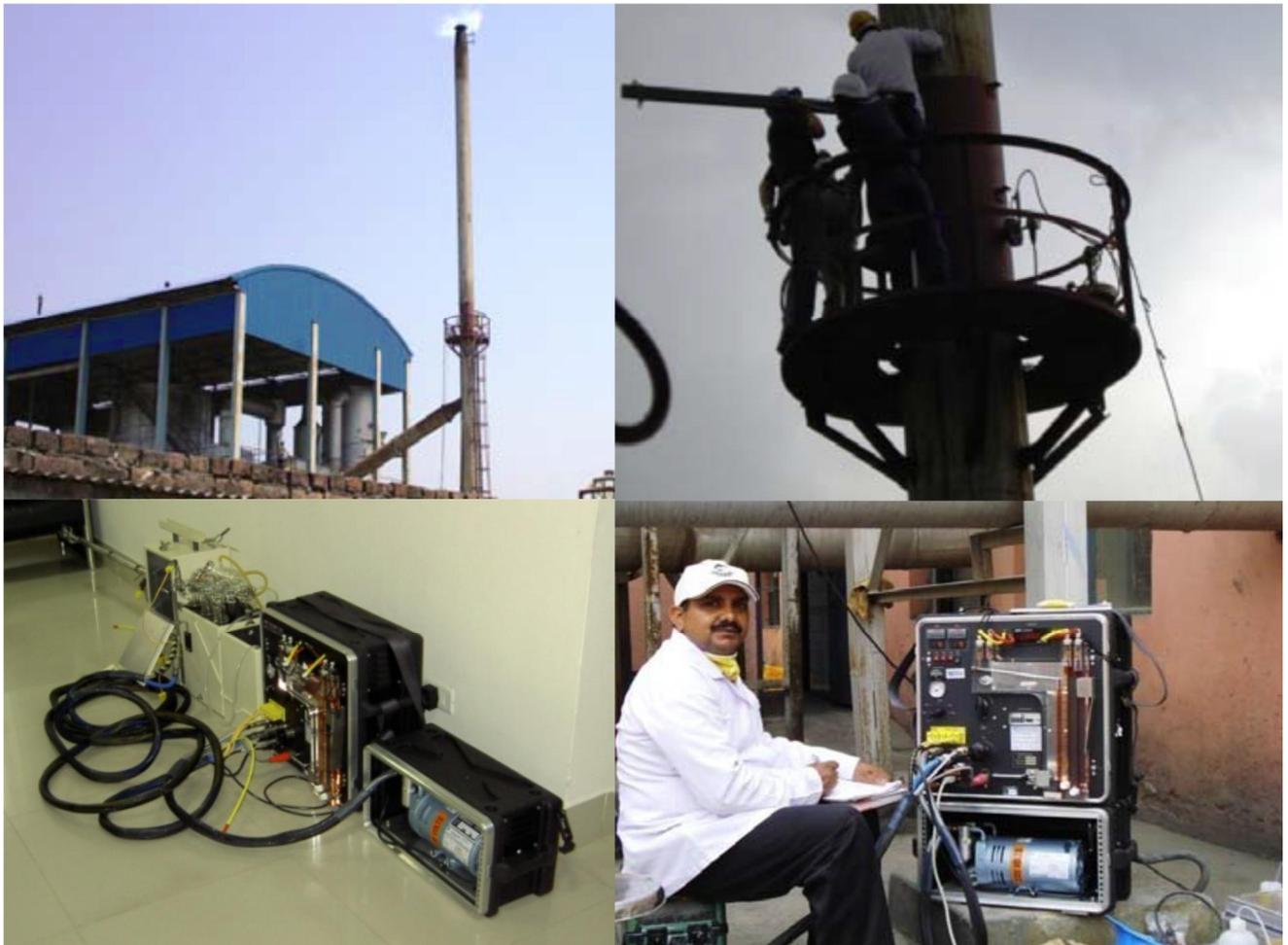
**Figure 3.** Process Waste Incinerator measurements. Isokinetic dioxin and furan sampling device. /15/
