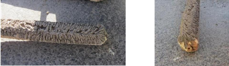
*Figure 3. Fouling of the probe after 7 months' operation in furnace.*
