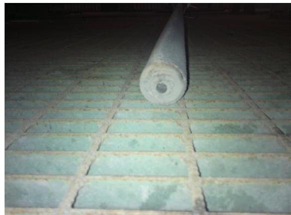
Figure 2. The sampling probe connection to the furnace (left), and the tip of the sampling probe in the beginning of the test (right).
