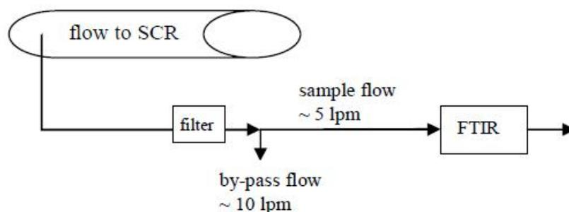
Figure 1. Ammonia sampling arrangement in inter-turbine SCR application.
