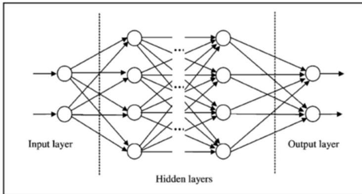
Figure 2. Layout of an artificial neural network with input layer, hidden layers and output layer /6/.
