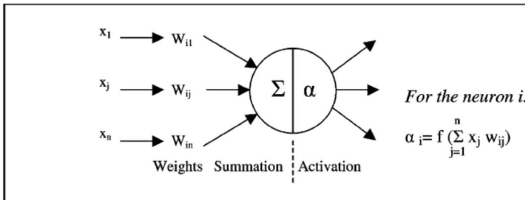
Figure 3. Processing of input information  $x_i$  to output  $a_i$  in a single node /6/.
