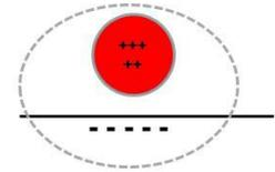
*Particles drift* in electric field. This can be used for particle collection, but it can also cause unwanted particle losses.
