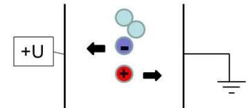
Insulated parts of *transportation lines* collect particles due to diffusion that then get charged. Accumulation of charge creates an electric field that finally prevents charged particles penetration through tube.
