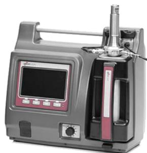
In High Temperature ELPI+ the detector part (Charger-Impactor assembly) is removed from its normal housing and placed into a separate heating unit:
