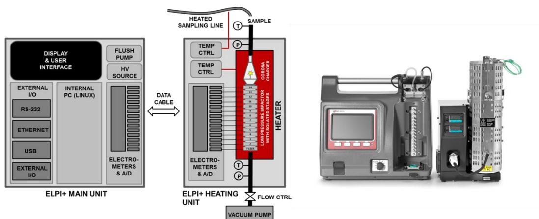
Heating unit contains the impactor and charger heater, insulation, temperature controls and a separate electrometer unit measuring the currents from the heated impactor. From there the measurement signals are transferred to the actual ELPI+ unit using a data cable. Further data processing and calculations are performed like in the normal ELPI+ measurement.
