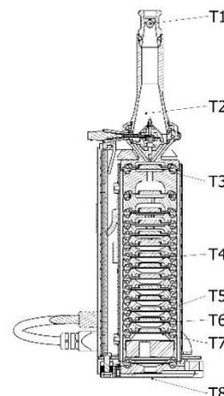
Starting from the room temperature impactor it takes approximately 4 hours until the temperatures are stabilized. Also due to heat losses and air gap between the impactor and its heater the impactor internal temperatures are slightly lower than the heater setpoint. However the actual impactor temperatures reach 150 degrees C which is enough to prevent condensation and nucleation in most cases.
