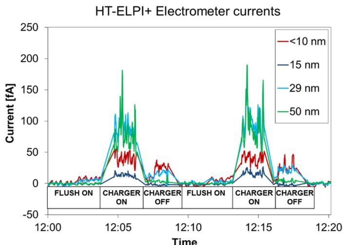
The result indicates clearly that the signal caused by the smallest particles (sub-10 nm particles, red line) is almost unaffected by the ELPI+ charger, meaning that these particles are highly charged already in the tailpipe. This results has two important meanings:
