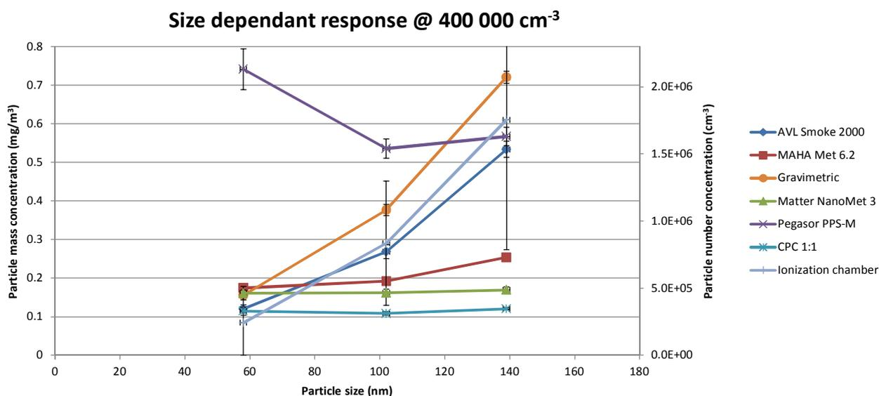
**Figure 10.** Particle size dependant response at particle concentrations of  $4 \cdot 10^5 \text{ cm}^{-3}$ . Light scattering instruments (AVL and MAHA) measuring only mass concentration are plotted against the left y-axis and the electrical sensors (Matter, Pegasor and ionization chamber) are plotted against the right y-axis. Standard deviation shown as error bars.
