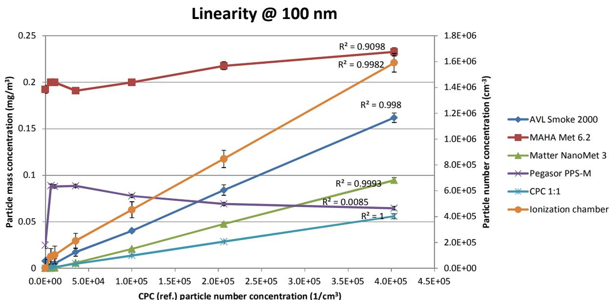
**Figure 6.** Linearity of measurement instruments for 100 nm soot particles. Light scattering instruments (AVL and MAHA) measuring only mass concentration are plotted against the left y-axis and the electrical sensors (Matter, Pegasor and ionization chamber) are plotted against the right y-axis. Standard deviation shown as error bars. The goodness of linear fit is shown as  $R^2$ .
