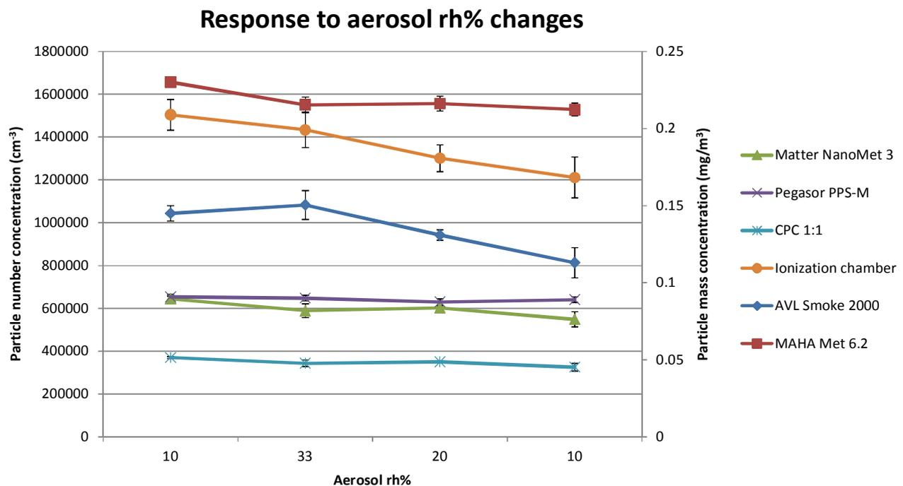
**Figure 13.** Effect of aerosol relative humidity measured at a particle concentration of  $4 \cdot 10^5$  and particle size 100 nm. Light scattering instruments (AVL and MAHA) measuring only mass concentration are plotted against the right y-axis and the electrical sensors (Matter, Pegasor and ionization chamber) are plotted against the left y-axis. Standard deviation shown as error bars.
