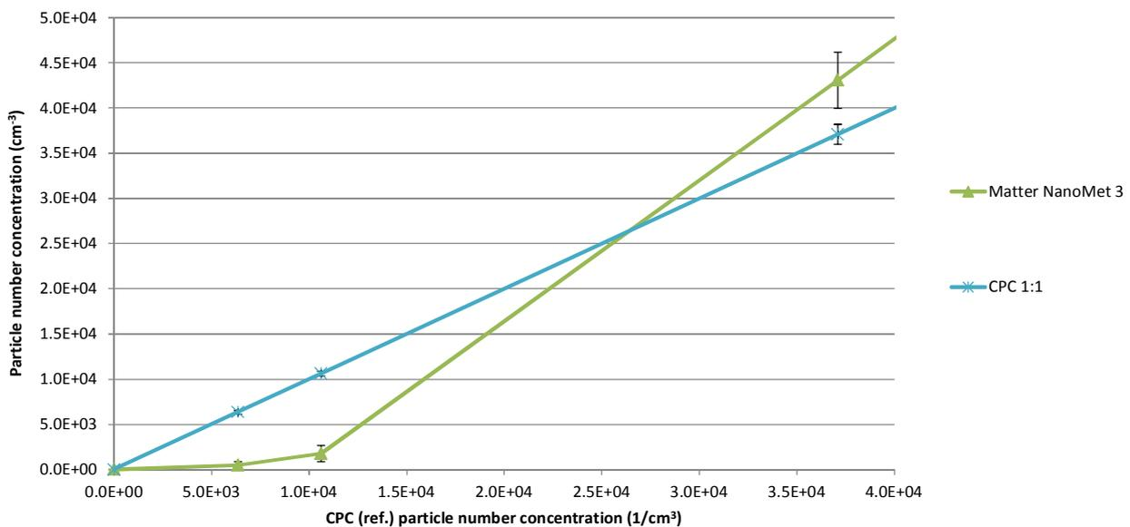
**Figure 3.** Linearity of Matter instrument for 40 nm soot particles and concentrations below  $4 \cdot 10^4 \text{ cm}^{-3}$ . Standard deviation shown as error bars.
