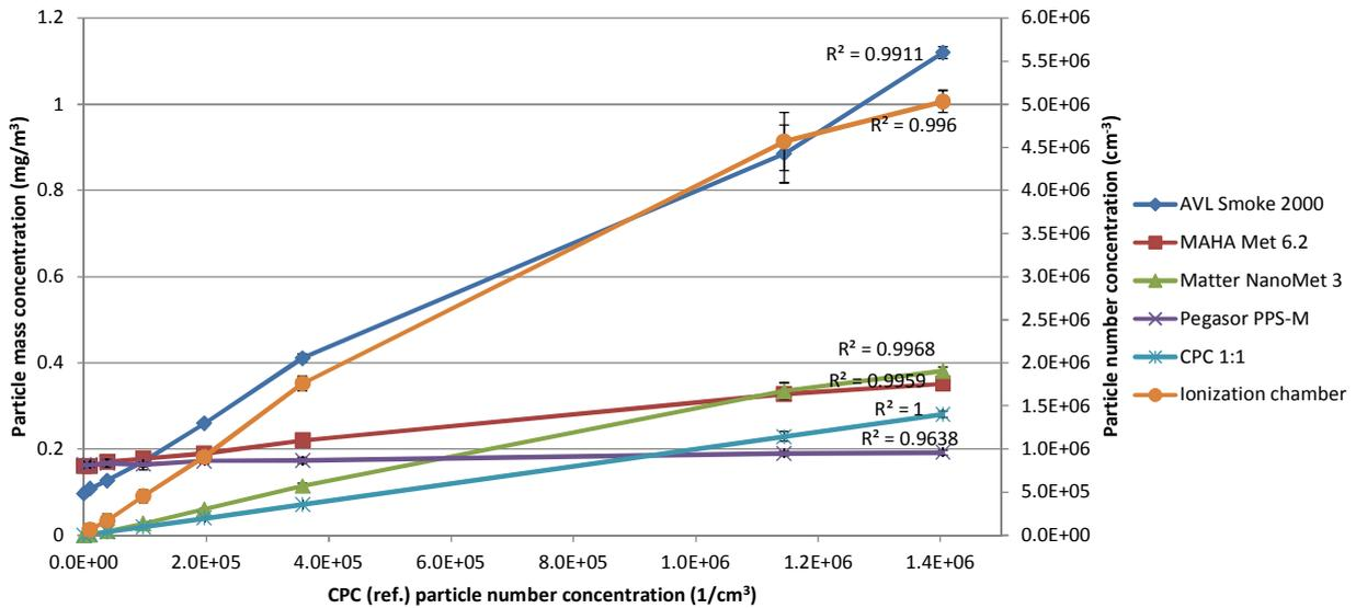
**Figure 8.** Linearity of measurement instruments for 150 nm soot particles. Light scattering instruments (AVL and MAHA) measuring only mass concentration are plotted against the left y-axis and the electrical sensors (Matter, Pegasor and ionization chamber) are plotted against the right y-axis. The goodness of linear fit is shown as  $R^2$ . Standard deviation shown as error bars.
