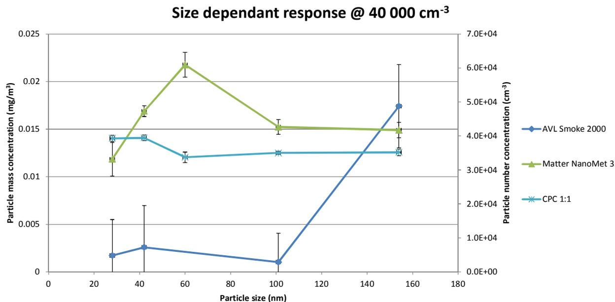
**Figure 12.** Particle size dependant response at particle concentrations of  $4 \cdot 10^4 \text{ cm}^{-3}$ . AVL instrument measuring mass concentration is plotted against the left y-axis and the Matter instrument is plotted against the right y-axis. Standard deviation shown as error bars.
