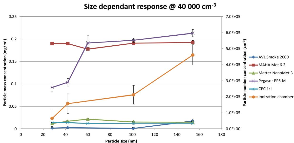
**Figure 11.** Particle size dependant response at particle concentrations of  $4 \cdot 10^4 \text{ cm}^{-3}$ . Light scattering instruments (AVL and MAHA) measuring only mass concentration are plotted against the left y-axis and the electrical sensors (Matter, Pegasor and ionization chamber) are plotted against the right y-axis. Standard deviation shown as error bars.
