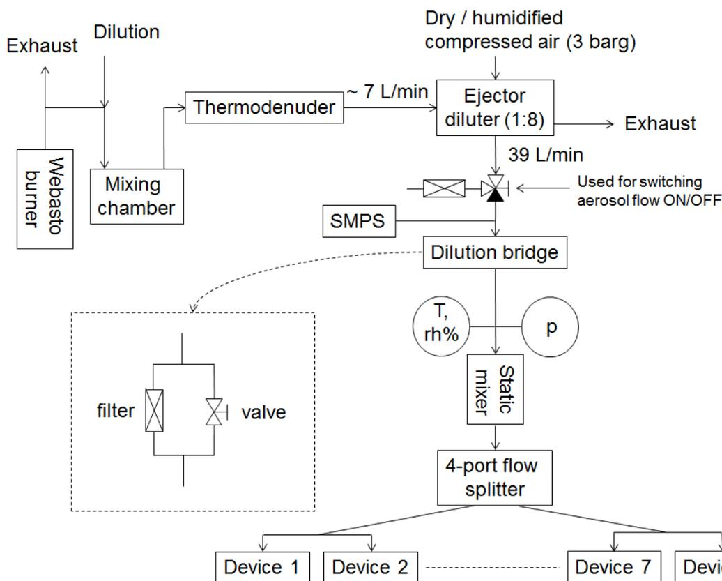
**Figure 1.** Experimental setup used for evaluating performance of particle measuring instruments.
