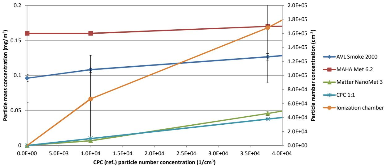
**Figure 9.** Linearity of measuring instrument responding to 40 nm soot particles and concentrations below  $4 \cdot 10^4 \text{ cm}^{-3}$ . Light scattering instruments (AVL and MAHA) measuring only mass concentration are plotted against the left y-axis and the electrical sensors (Matter, Pegasor and ionization chamber) are plotted against the right y-axis. Standard deviation shown as error bars.
