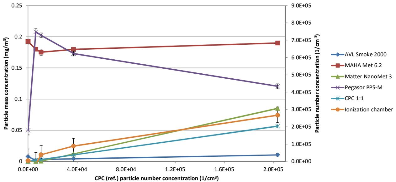
**Figure 2.** Linearity of measurement instruments for 40 nm soot particles. Light scattering instruments (AVL and MAHA) measuring only mass concentration are plotted against the left y-axis and the electrical sensors (Matter, Pegasor and ionization chamber) are plotted against the right y-axis. Standard deviation shown as error bars.
