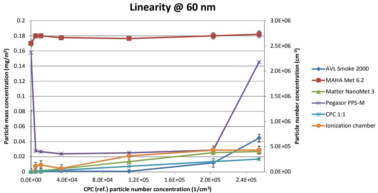
**Figure 4.** Linearity of measurement instruments for 60 nm soot particles. Light scattering instruments (AVL and MAHA) measuring only mass concentration are plotted against the left y-axis and the electrical sensors (Matter and Pegasor) are plotted against the right y-axis. Standard deviation shown as error bars.
