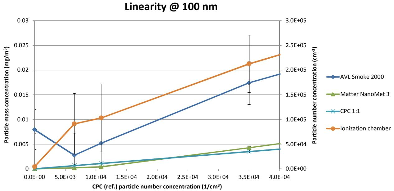
**Figure 7.** Linearity of measurement instruments responding to 100 nm soot particles with concentrations below  $4 \cdot 10^4 \text{ cm}^{-3}$ . AVL mass concentration is plotted against the left y-axis and the Matter and ionization chamber number concentrations are plotted against the right y-axis. Standard deviation shown as error bars.
