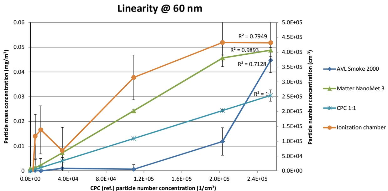
**Figure 5.** Linearity of measurement instruments responding to 60 nm soot particles. AVL mass concentration is plotted against the left y-axis and the Matter and ionization chamber number concentrations are plotted against the right y-axis. The goodness of linear fit is shown as  $R^2$ . Standard deviation shown as error bars.
