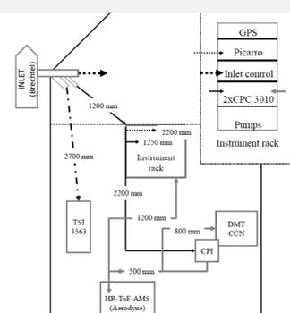
Figure 2. Schematics of instruments inside the Short SC-7 Skyvan airplane. Instruments onboard on first flights measured aerosol chemistry (SP-AMS), aerosol cloud activation properties (CCN counter), aerosol scattering (Nephelometer), aerosol total concentration (CPC) and greenhouse gas concentrations (Picarro). Inlet controller unit kept the inlet flow isokinetic.
