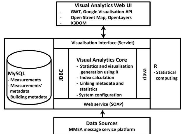
Figure 3. Prototype architecture
