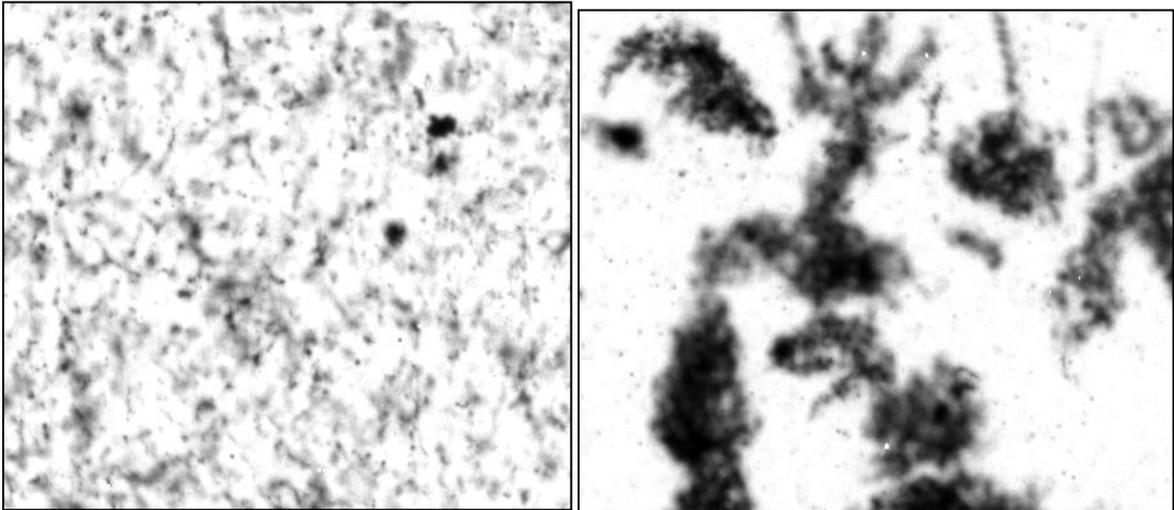
**Figure 2.** Original image of activated sludge floc (left) and conditioned activated sludge flocs (right).
