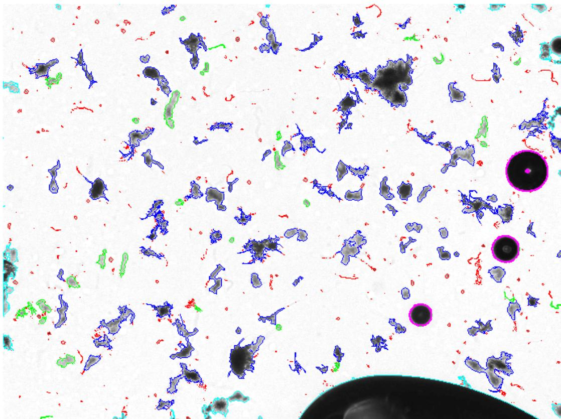
**Figure 4.** An example of object classification in image preprocessing. Boundaries of objects touching image border are colored in cyan, out-of-focus objects in green, small debris in red, air bubbles in magenta and accepted objects in blue.
