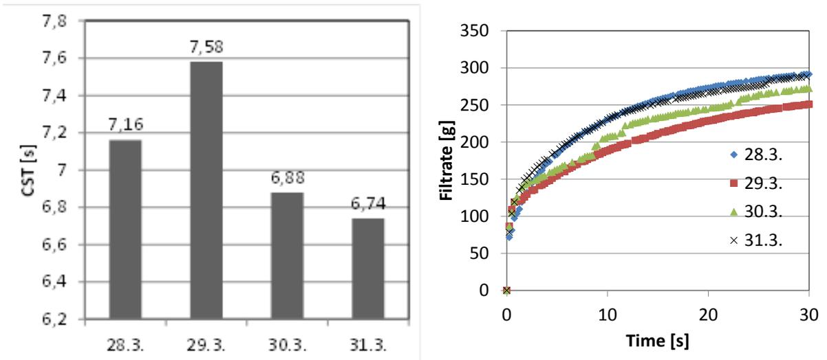
**Figure 2.** Dewatering properties of activated sludge in March 2011.
