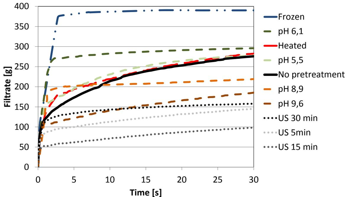
**Figure 5.** Filtration properties of pre-treated activated sludge flocs.
