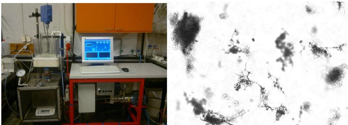
**Figure 1.** Mofi measurement environment (left) and captured floc image (right).
