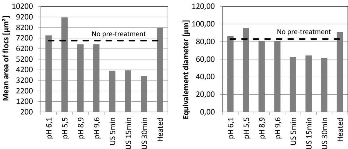
**Figure 7.** Size of pre-treated activates sludge flocs.
