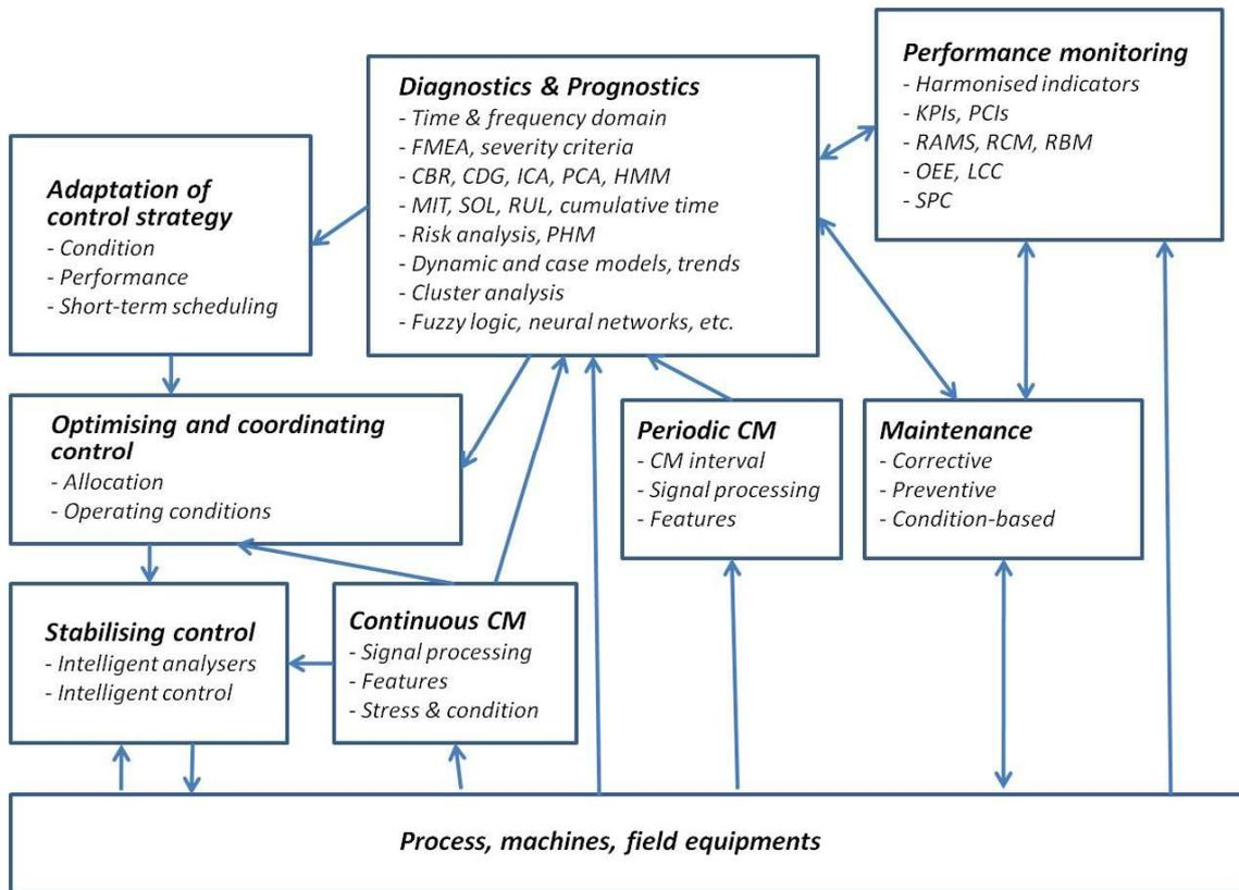
Figure 5. Integrated control and condition-based maintenance <sup>(13)</sup>.
