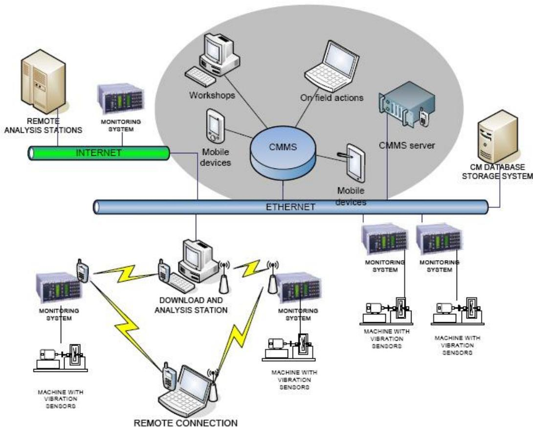
**Figure 1. Typical architecture of maintenance information system<sup>(1)</sup>.**
