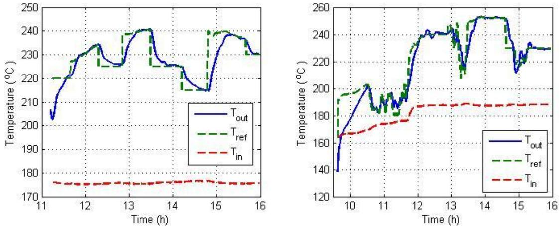
**Figure 3** Test results of the LE controller: (a) a fairly clear day, (b) a cloudy day.
