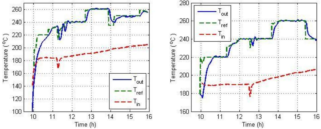
**Figure 4** Test results of the LE controller on a fairly clear day including a load disturbance: (a) without special actions, (b) delayed actions. Improved asymmetrical action is used in (b).
