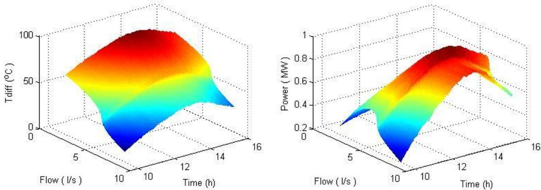
**Figure 5** Energy collection alternatives vs. oil flow and time: (a) temperature difference across the field, (b) collected power.
