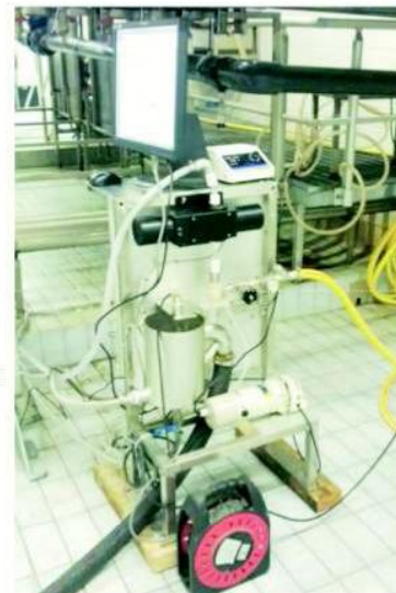
Fig. 1. Schematic illustration of floc measurement environment (MOFI) and MOFI at Viikinmäki waste water treatment plant.
