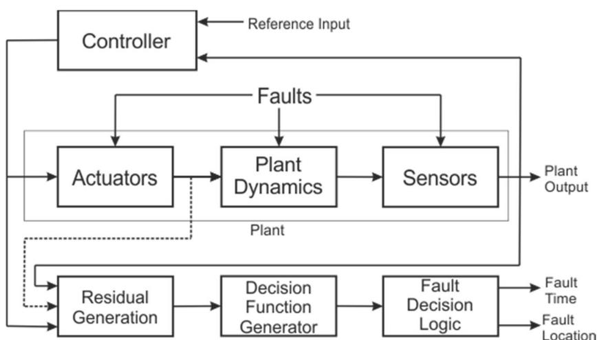
Figure 4. Conceptual scheme for model-based fault detection introduced by Frank (1990).
