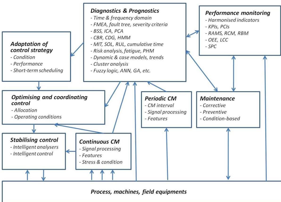
Figure 6. Integrated control and condition-based maintenance (Juuso 2013).
